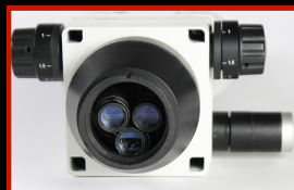
UltraZOOM-6 showing 3 zooming objectives, one of which is dedicated to the camera
